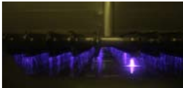
Plasma and Radicals Within the AquaPure Reactor
